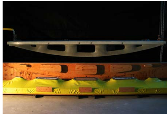
Fig. 2 Concrete truss cast at the University of Manitoba, with the timber and fabric formwork shown below in two seperated parts
